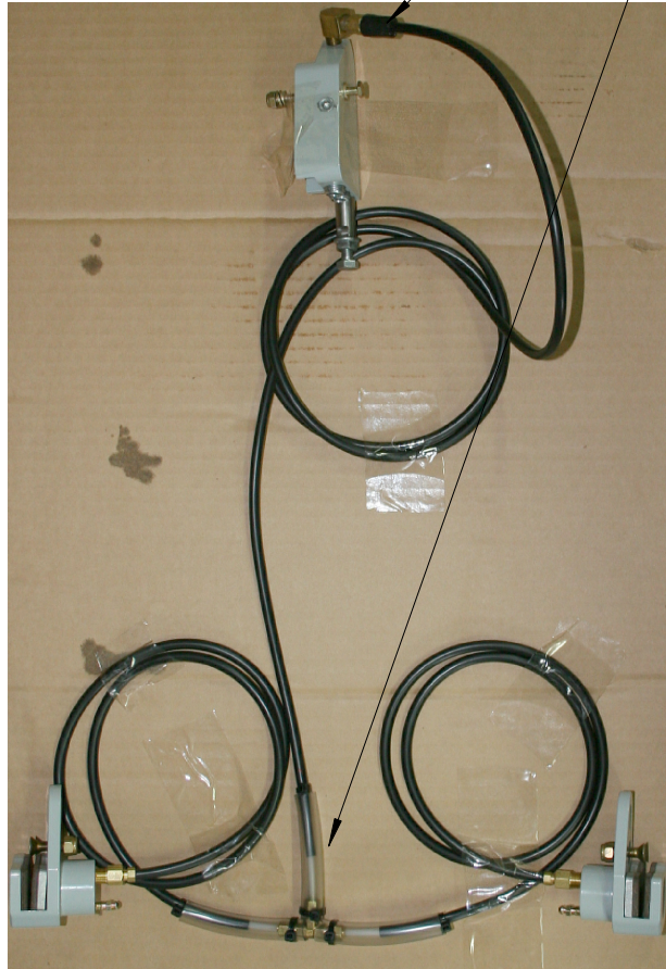
PHOTO SHOWS BRAKE LINE ASSEMBLY (PLUS OTHER PARTS TO SHOW ASSEMBLY CONTEXT)
